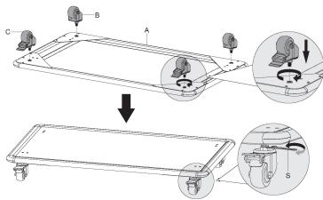
Each caster can be adjusted independently for fine tuning Slightly turn the nut to lower or raise the base.
